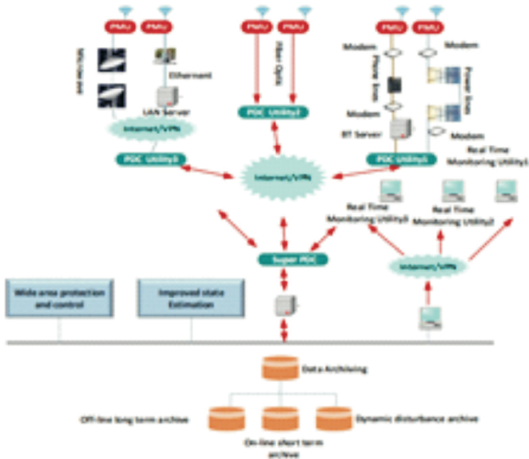
Figure 5: WAMC Architecture,(Terzija et al., 2011)
