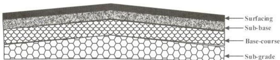
Fig. 1: Typical pavement stratum for a heavily traveled road
