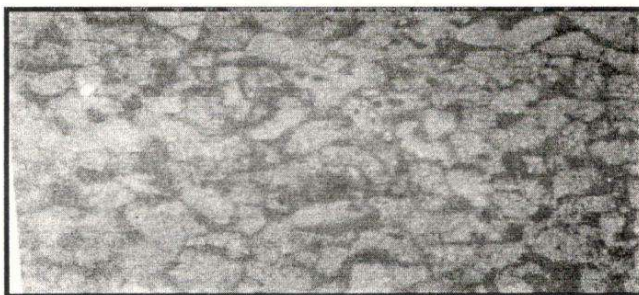
Plate B: Normalised ST60-2 Aladja structural steel. The structure consists of pearlite (Dark gray) and ferrite matrix (White). (X200).
