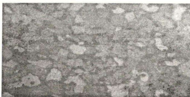
Plate G: ST60-2 Aladja Structural steel brine quenched and tempered at 450°C. The structure shows tempered martensite (Grey) with patches of ferrite. (x200).
