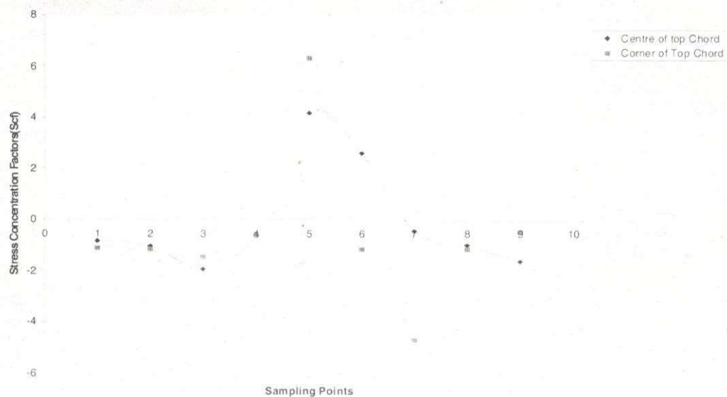
Figure 7. Effect of geometry on Stress conc.Factors(Scf) for 70 mm gap Joint.
