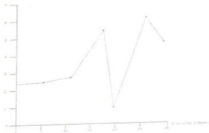
Fig. 4 Graph of experimental variogram in east-west direction of Ekarin-Ado calcite deposit
