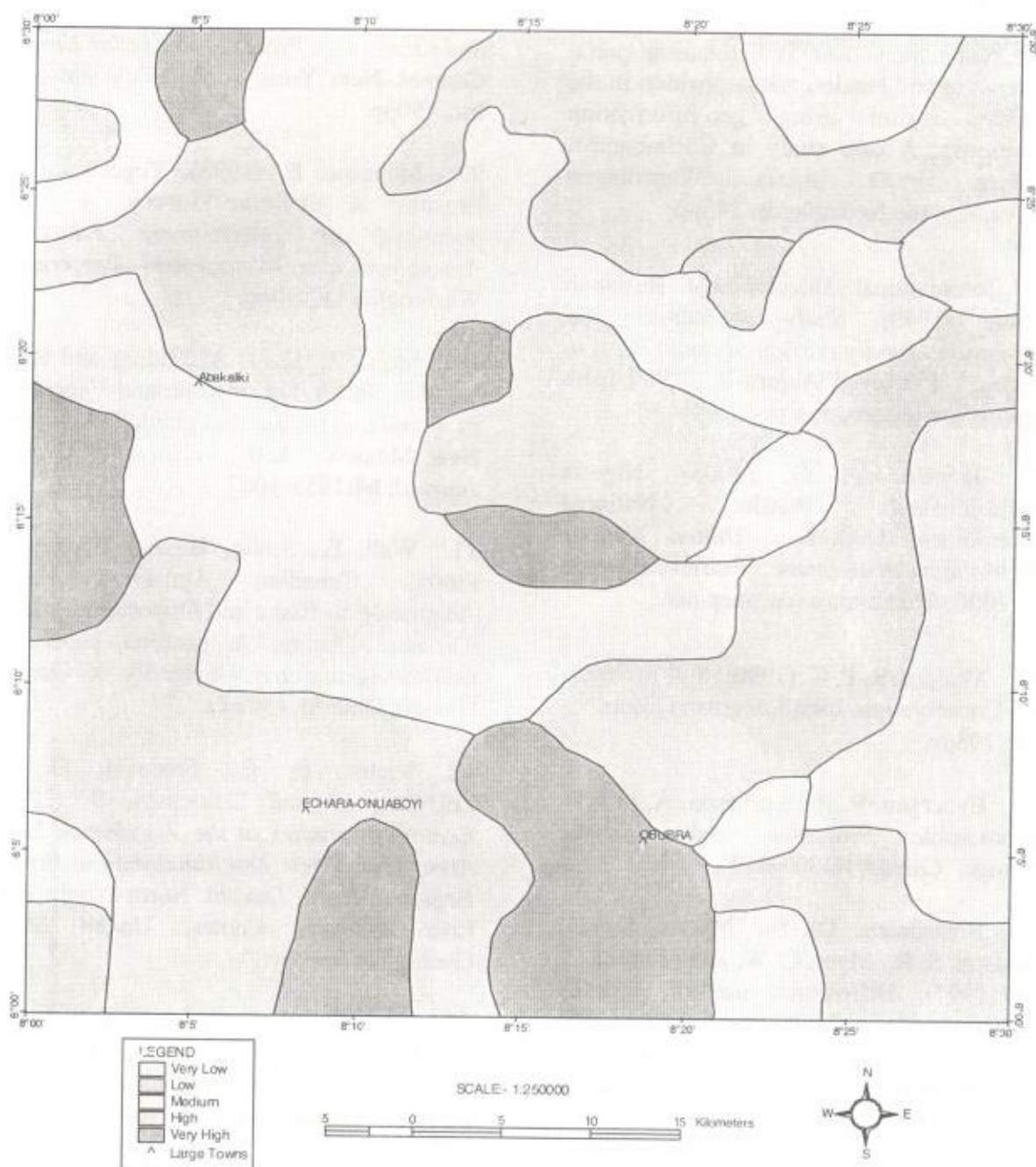
Fig. 9: Potential Soil Erodibility
