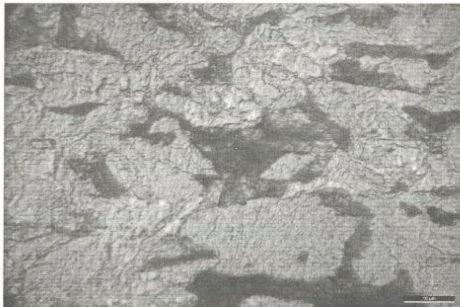
Plate 4: Photomicrograph showing the Microstructure of P/70%/740 0 C, 30mins/H 2 O. The structure reveals pearlite (gray coloured phase) with dispersed Islands of Martensite (dark phase).
