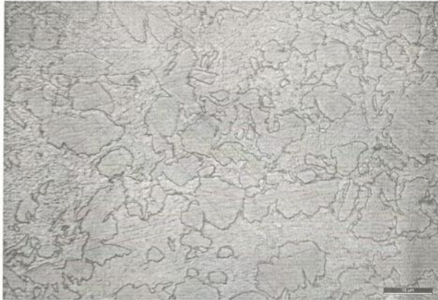
Plate 3: Photomicrograph showing the Microstructure of P/70%/740 0 C, 15mins/H 2 O. The structure reveals recrystallized grains of pearlite
