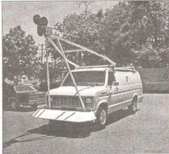
Figure 1: Data Collection Vehicle for 35mm Analogue Continuous Film Technology
